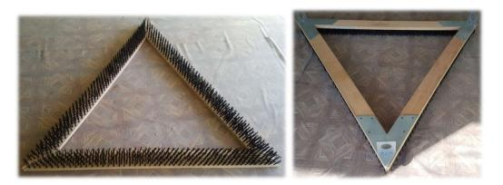
The length of one side of triangular brush is 1500mm and its weight is 15 kg. The product is delivered to the cargo in disassembled form in dimensions of 1500x100x320mm. The brushes have a diameter of 3mm and a length of 80mm and are hammered into kiln-dried beech wood with a thickness of 25mm and a width of 100mm, which is resistant to stretching. The connection parts are made of 4mm DKP steel sheet.
