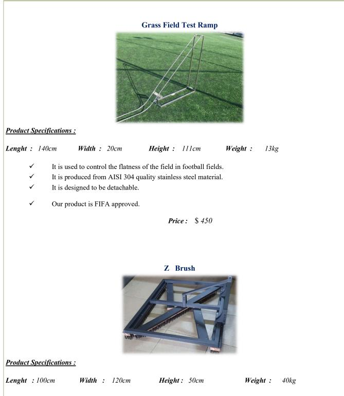
Thanks to 2 flat and 3 cross placed brushes, it provides successful maintenance in the field. The sheets to which the brushes are attached are made of 2mm 1st Class ST37 steel material, and the frame that turns around is made of 40x40 profile. The brushes have a diameter of 3mm and a length of 80mm and are hammered into kiln-dried beech wood with a thickness of 25mm and a width of 100mm, which is also resistant to stretching. It can be attached to the ATV vehicle or to the back of a tractor.
